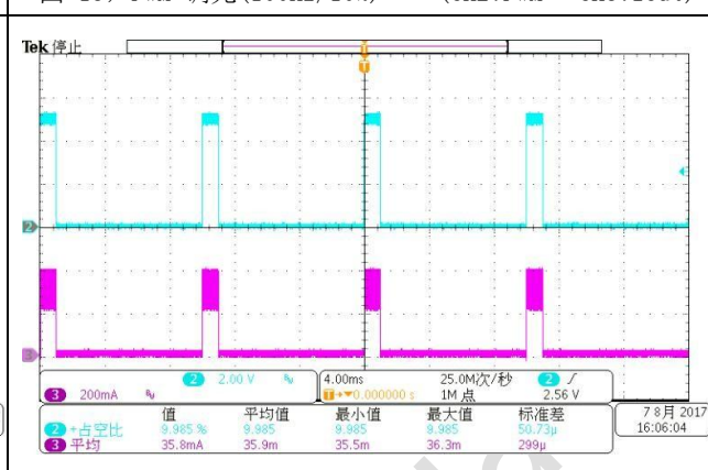
图 13, PWM 调光(100Hz/10%) (CH2:PWM CH3:Iout)
