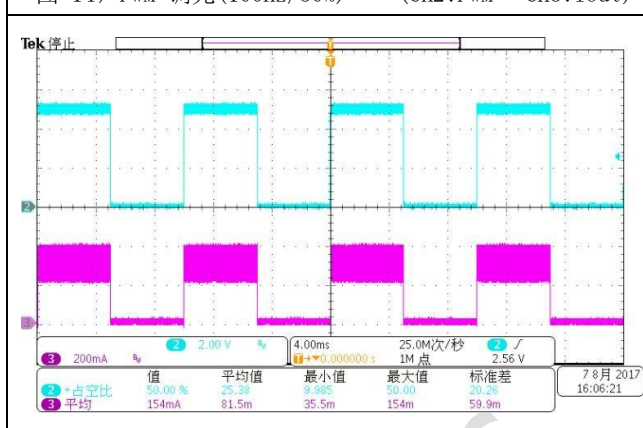
图 14, PWM 调光(100Hz/50%) (CH2:PWM CH3:Iout)
