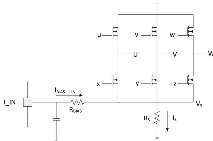
$$V_{I\_FB} = (V_S \times 8) + (I_{BIAS\_I\_IN} \times R_{BIAS}) \quad (1)$$
